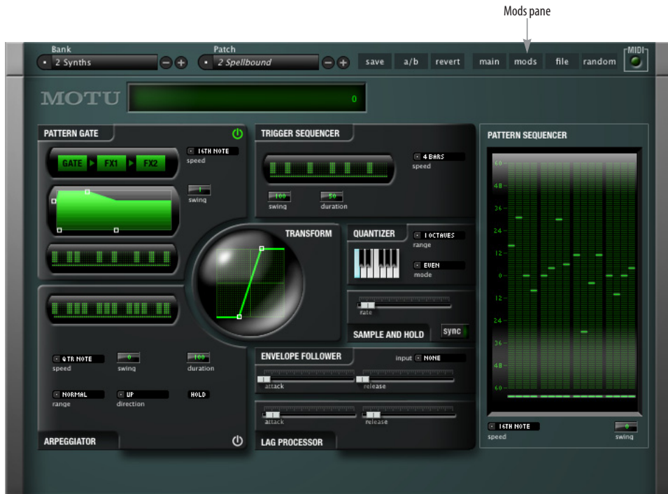
Figure 7-24: The Mods pane provides a Pattern Gate, Arpeggiator, Envelope Follower, Pattern Sequencer, Transform, Quantizer, Sample and Hold, Lag Processor and Trigger Sequencer.
