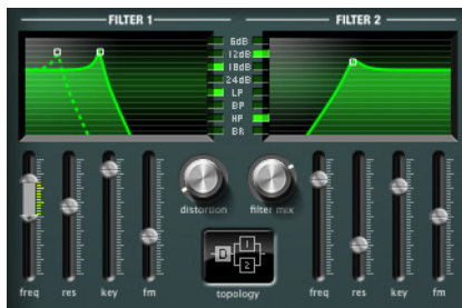
Figure 7-16: the filter section.
